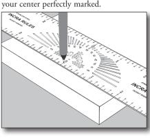
You'll also find your centering rule handy for laying out a series of measurements on either side of any known starting point Simply scribe a line at your starting point, align the zero with your mark, then twist your pencil through the hole at each of the desired measurements.
