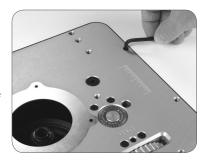
The PRL-V2 also features a brake. For most routers, the brake isn't necessary. However if you experience vibration while routing, the brake will prevent the bit height from changing on its own. A 1/8" hex key is supplied for the brake. **DO NOT OVER TIGHTEN THE BRAKE.** A little pressure is all that is required.
