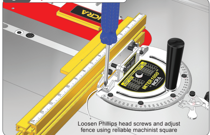
Fig. 8 Square Fence to Blade
